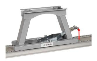
To remove the seat leg, press the locking lever slightly downwards. Pull the lock forward, then lift the locking lever upwards to release.
