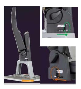
Pull the adjustment lever forwards, then rotate the seat (using both hands) to the desired position. When the rotation position is reached (quarter turn), the lever locks back into the home position under spring tension.
