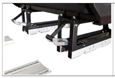
The SL3 bench must be pushed into the vehicle by **at least two people** and placed on the aluminium profiles.
