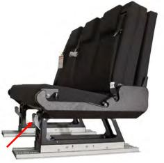
Move the bench to the desired position and then remove the locking pins.
