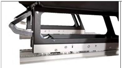
After placing it on the aluminium profile, the bench must be pushed until it clicks into the floor profile.
