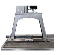
Now your EasyLeg seat leg is engaged on the aluminium system floor.
