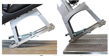
Insert the wheels into the holes in the floor rail. If you have chosen the EasyLeg seat leg without wheels, insert the rear mushroom head screw into the floor profile. This positions the mushroom head screws and makes it easier to insert them into the rail.
