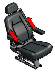
The angle of inclination of the armrests can be set to the desired position by turning the handwheel.
