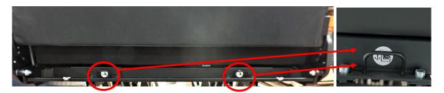
The Top-Tether attachment eyelets are located on the back of the bench, below the back cushion on the rear leg attachment.
