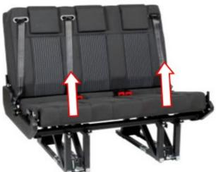
4. Fold the seat section upwards
