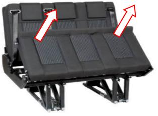
**6.** Pull the release lever upwards while holding the retaining lug (see also warning note danger of crushing)
